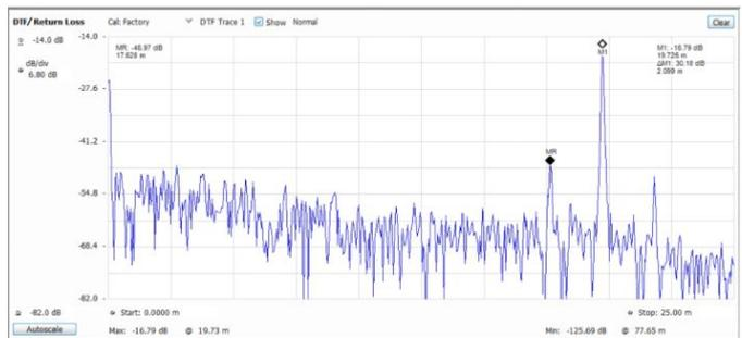
电缆的回波损耗与距离关系，其中插入了一个桶状连接器和一条扩展电缆。The point at M2 (17.638 m, MR) is the barrel connector and the point marked by M1 at 19.725 m is the end of the cable.
