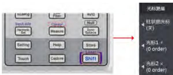
图 17.7 柱状图光标测量菜单
