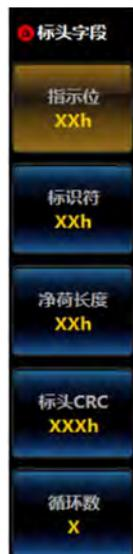
图11.164 FlexRay 总线标头字段触发二级菜单
