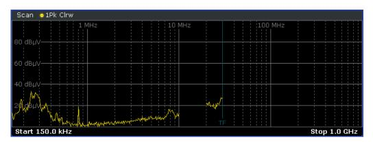
Figure 9-7: Scan on selected frequencies showing gaps in the trace
