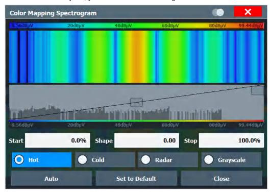
Figure 11-4: Spectrogram with (default) linear color curve shape = 0
