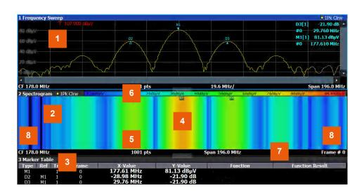
Figure 11-3: Screen layout of the spectrogram result display
