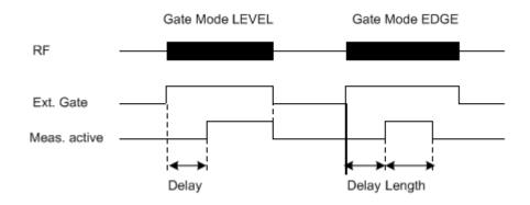
Figure 10-9: Effects of Gate mode, Gate delay and Gate length
