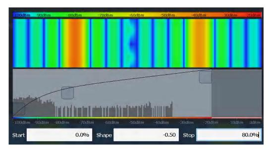
Figure 11-5: Spectrogram with non-linear color curve (shape = -0.5)
