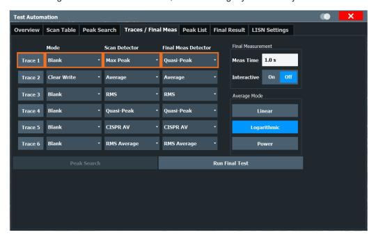
Figure 9-14: Overview of the Final Meas configuration
