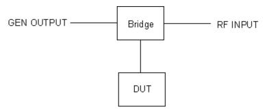
Figure 10-5: Test setup for reflection measurement
