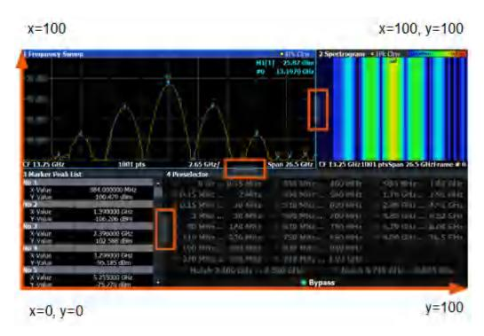
Figure 15-1: SmartGrid coordinates for remote control of the splitters
