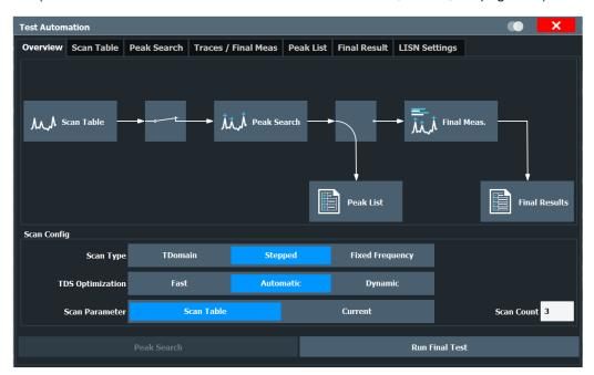
Figure 9-8: Overview of the test automation process
