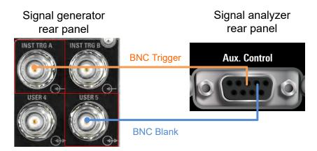
Figure 10-2: TTL connection for an R&S SMW generator
