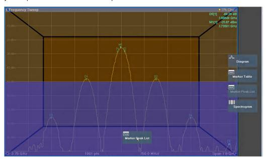
Figure 6-5: Moving a window in SmartGrid mode
