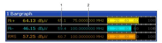
Figure 9-2: Screen layout of the bargraph result display with the max hold information
