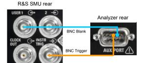
Figure 10-1: TTL connection for an R&S SMU generator
