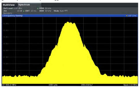
Figure 10-10: GSM signal with GATE OFF
