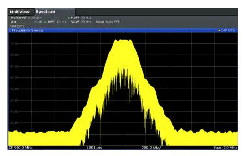
Figure 10-11: GSM signal with GATE ON
