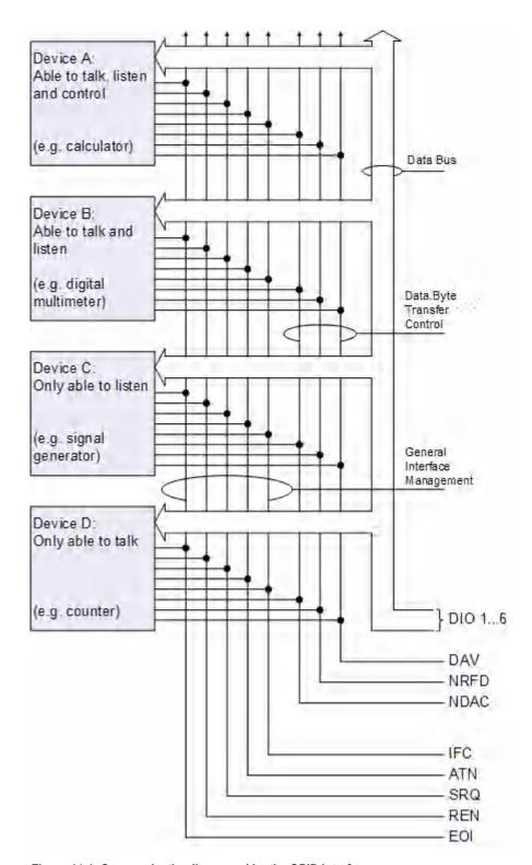
Figure 14-1: Communication lines used by the GPIB interface
