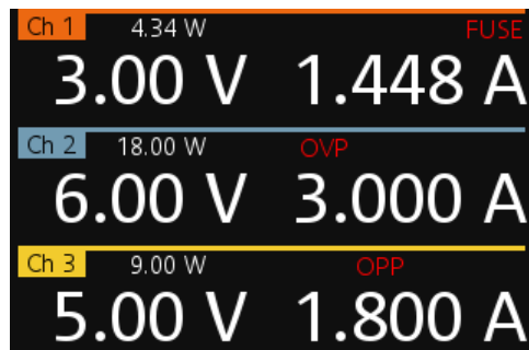
Figure 5-13: Indicator of OVP/OPP when tripped
