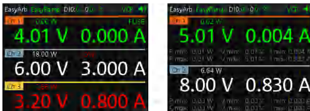
Figure 5-1: Screen layout for 3-channel or 2-channel instrument
