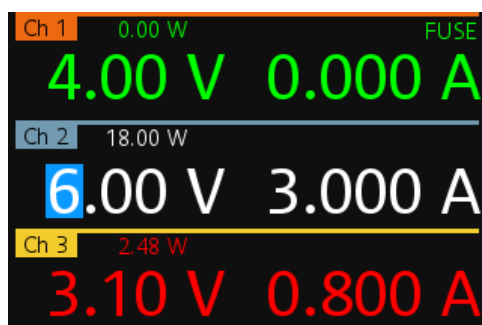
Figure 5-3: Color coding of operating condition
