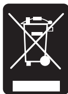
Fig. 1.4: Product labeling in accordance with EN 50419
