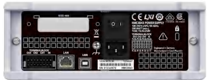
Fig. 1.2: Back panel R&S®HMC804x with connectors
