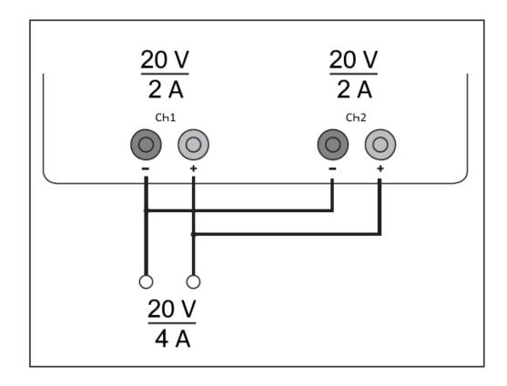
Figure 8-2: Example of parallel connection
