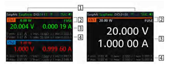
Figure 5-1: Screen layout of R&S NGA100 for two-channel and single channel display
