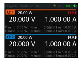
Figure 6-6: Fuse indicator on respective channel
