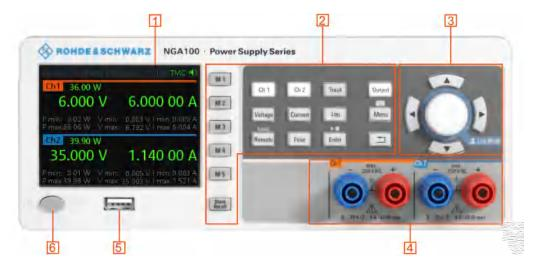
Figure 4-2: Front panel of R&S NGA100 with 2 channels
