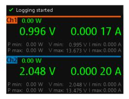
Toggle the [Log] key to stop data logging. The R&S NGA100 finishes the data logging. An indicator "Finish writing to usb" is displayed on the status bar.
