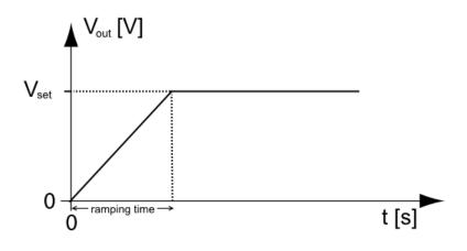
Figure 6-13: Ramping voltage output
