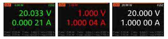
Figure 5-3: Color coding of difference operating conditions
