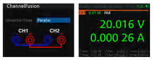
Figure 6-5: Parallel mode setting and output of one-channel display
