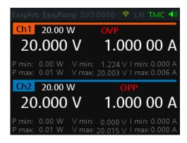
Figure 6-8: Indicator of OVP/OPP when tripped
