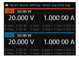
Press any of the memory keys ([M1],[M2], [M3], [M4], [M5]) to recall the instrument settings.
