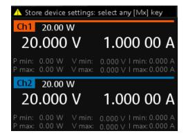
Press any of the memory keys ([M1],[M2], [M3], [M4], [M5]) to store the instrument settings.
