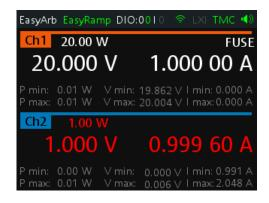
Figure 6-3: Output of Ch2 in CC mode
