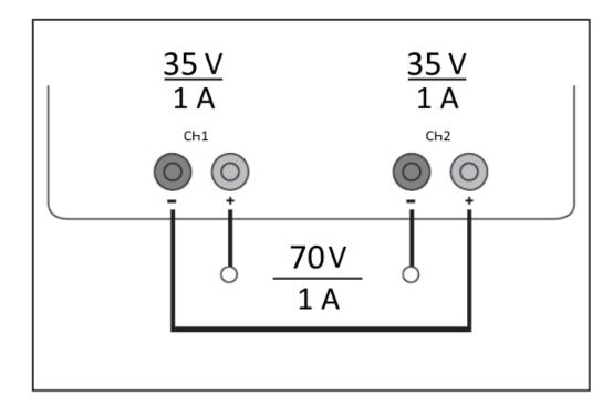
Figure 8-1: Example of series connection
