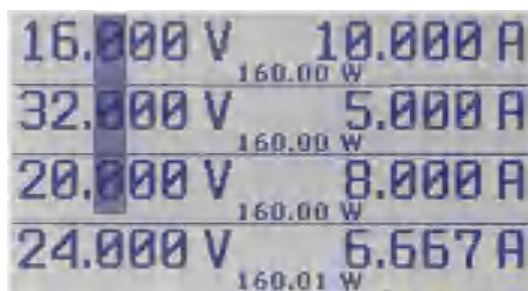
Figure 4-2: Changing the 100 mV position for three channels with the tracking function
