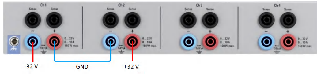
Figure 5-5: Example of a multi-quadrant connection
