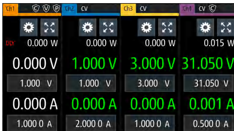
Figure 6-5: Delay text at channel display area
