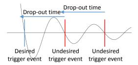
For the external trigger, the drop-out time defines a minimum duration that the input signal must stay below the trigger level before triggering again. The dropout time helps you stabilize triggering when the analyzer is triggering on undesired events.
