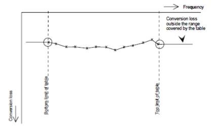
Figure 10-2: Conversion loss outside the band's frequency range
