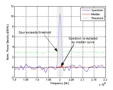
Figure 11-6: Spur detection and removal principle
