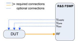
Figure 6-1: Typical test setup for basic noise measurements
