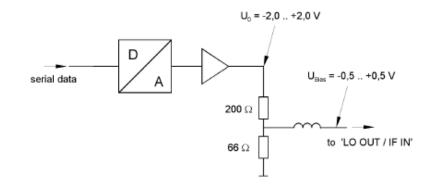
Figure 10-1: Bias circuit of the R&S FSWP
