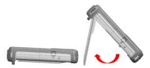
When laid out horizontally for operation from above, the R&S ZNH is tilted slightly due to the micro-stand at the back. This position provides the optimum viewing angle for the display.
