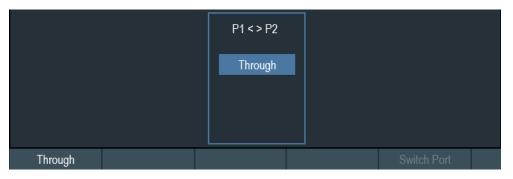
The R&S ZNH is now calibrated and a "(norm)" status is displayed next to the measurement format, i.e. **S21 (norm) Mag.** See Chapter 3.2.6, "Display Overview", on page 28.
