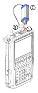
Figure 7-10: Calibration kit, R&S ZN-Z103
