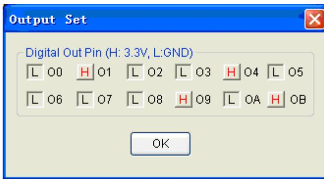
By selecting one pin, that digital output pin will output high level. Otherwise, the pin will output low level.
