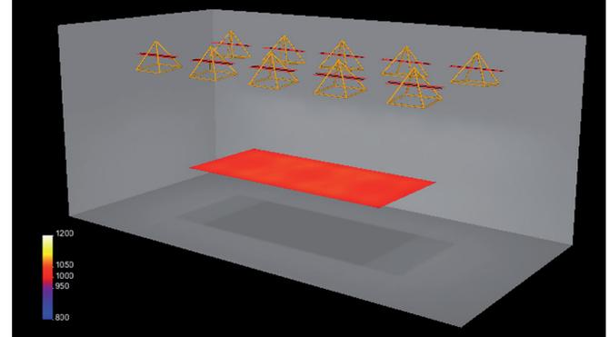
SolarConstant MHG 4000/2500 are often used for solar simulators integrated into climatic chambers. The tool of choice to determine thermal heating effects of solar radiation, such as fit and finish, dimensional stability or thermal transmission. Further to identify photodegradation effects of polymers and coatings such as change of color, gloss, haptics or physical strength. Further, testing PV module performance.
