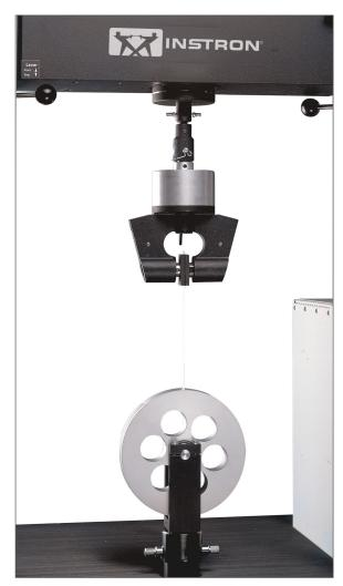
Rotating German wheel peel fixture
