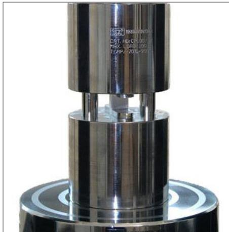
CP105787 Wyoming Modified Celanese Compression Test Fixture
