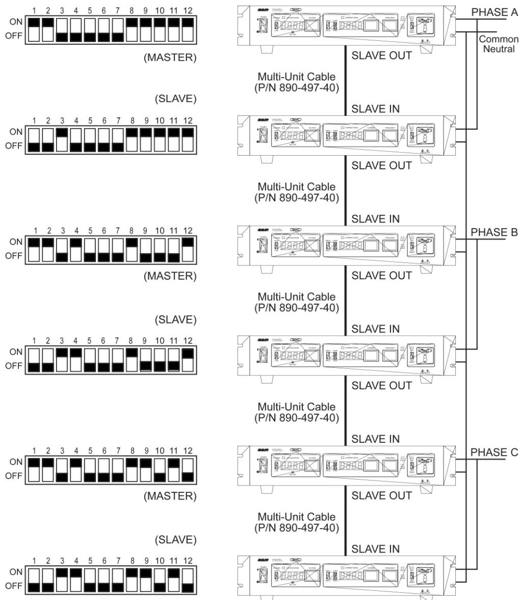
Figure 4-5. Dipswitch Settings for 3-Phase, 2-Paralleled Each, Configuration
