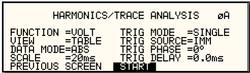
Figure 4-10: HARMONICS/TRACE ANALYSIS Screen
