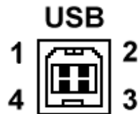
Figure 3-11: USB Connector Pin Orientation.
