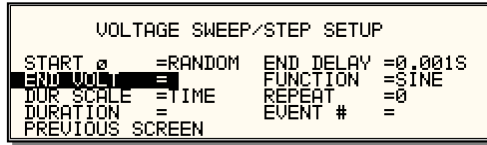
Figure 4-13: VOLTAGE SWEEP/STEP SETUP Screen
