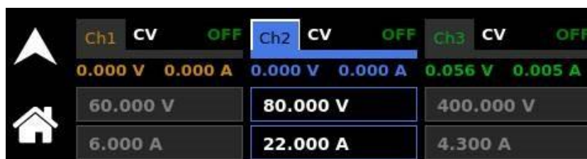
Figure 3-21: Dashboard Screen – Channel 2
