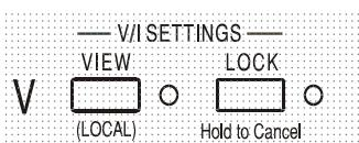
The set voltage and current limit are always shown when the output is off but can also be viewed when the output is on by pressing the VIEW key; the VIEW lamp is lit whilst the VIEW key is pressed.
