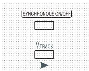
Pressing  $V_{\text{TRACK}}$  selects voltage tracking mode. The two outputs remain electrically isolated but the Voltage controls of Output 1 (the Master) set an identical voltage on Output 2 (the Slave).
