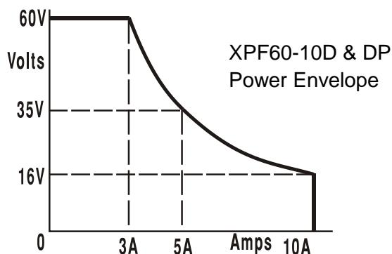
The power envelope is set to give 60V/3A, 35V/5A and 16V/10A under all supply conditions (both outputs loaded); at lower output voltages the output power is restricted by the 10A current maximum.
