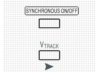
The SYNCHRONOUS ON/OFF key is in addition to the individual OUTPUT switches and permit both outputs to be turned on or off synchronously with a single key press. Since this key turns both outputs on or off with alternate presses it is necessary for both outputs to be in the same state (i.e. both on or both off) before the key is used. Pressing the key with one output on and one output off will have no effect.
