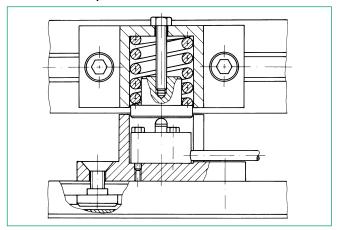
Overload of the load cell is impossible due to a suitable spring. When the units are locked the spring will transfer not more load to the cell than the measuring range can cope with.
