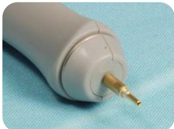
MCP-6 Probe Set with Coaxial Pins Installed
