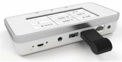
Connect the Bluetooth adapter to a SENSOR port on the base unit. A gray Bluetooth status symbol appears in the upper right corner of the screen.
