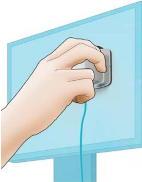
**Luminance:** Place the connected sensor with the aperture centered on the area you want to measure, and with luminance selected on the sensor wheel.
