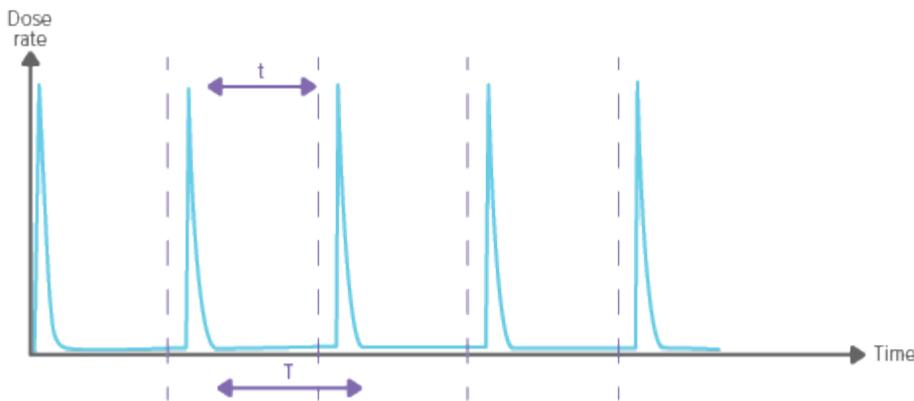
Stop delay setting ( $t$ ) shorter than the time between pulses ( $t < T$ ), will result in many short measurements (one for each pulse).
