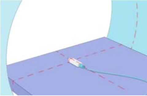
For kVp measurements, use an R/F sensor. Position it flat on the table and expose without rotation, using scout, tomogram or topogram mode. Use no or slowest table movement.
