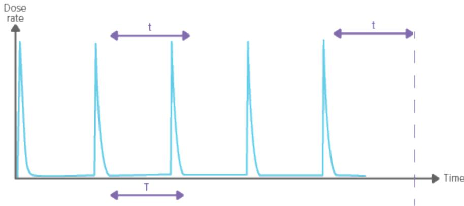
Stop delay ( $t$ ) setting longer than the time between pulses ( $t > T$ ), will result in one long measurement. Note that you have to wait as long as the stop delay setting ( $t$ ) after the last exposure before the measurement ends and values will be displayed.
