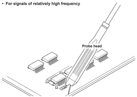
Select an attachment according to the circuit to be tested (straight pin, angle pin, spring type straight pin, spring type angle pin).
