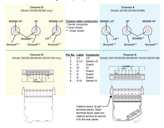
Figure 23: Input/output connectors
