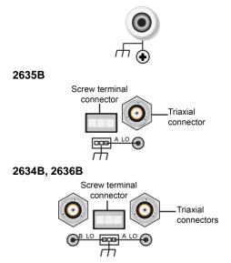
Ground terminal for connection output HI or LO to chassis ground. Ground screw for connections to chassis ground.
