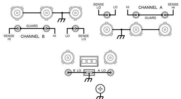
For the 2601B, 2602B, 2604B, 2611B, 2612B, and 2614B, there is a low-noise chassis ground banana jack that can be used as a common signal ground point for input and output LOs. This low-noise signal ground banana jack is connected to the chassis through a frequency variable resistor (FVR).
