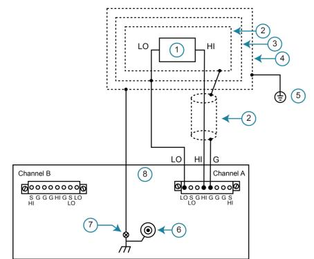
Figure 36: Connections for noise shield, safety shield, and guarding
