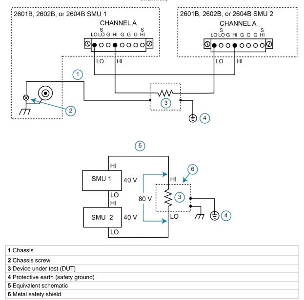
Figure 31: Safety shield for hazardous voltage combining two 2601B, 2602B, or 2604B channels
