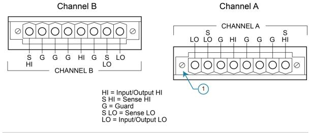
1 Captive screw. Each terminal block uses two captive screws to secure it to the rear panel.
