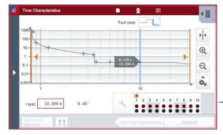
Perform multiple test shots at different output values. The results can be easily compared with the relay's nominal characteristic.
