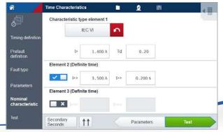
Specify the relay's nominal characteristic to be used as a reference. Choose from inverse and definite time characteristics. (Available for fault types I L-E, I L-L and I 3Ph)
