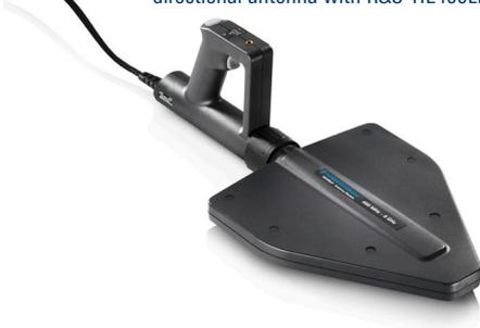
The R&S®HE400MW antenna handle operates from 20 MHz to 20 GHz. It supports the R&S®HE400VHF, R&S®HE400UWB, R&S®HE400LP, R&S®HE400CEL, R&S®HE400SCB and R&S®HE400SHF antenna modules and is compatible with the R&S®Spectrum Rider FPH handheld spectrum analyzer (models .13/.23/.26/.36), the R&S®FSH13 and R&S®FSH20 handheld spectrum analyzers and the R&S®CableRider ZPH cable and antenna analyzer (model .12).
