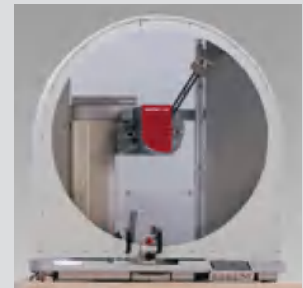
Fig. 4: HIT50P electrically interlocked safety device
