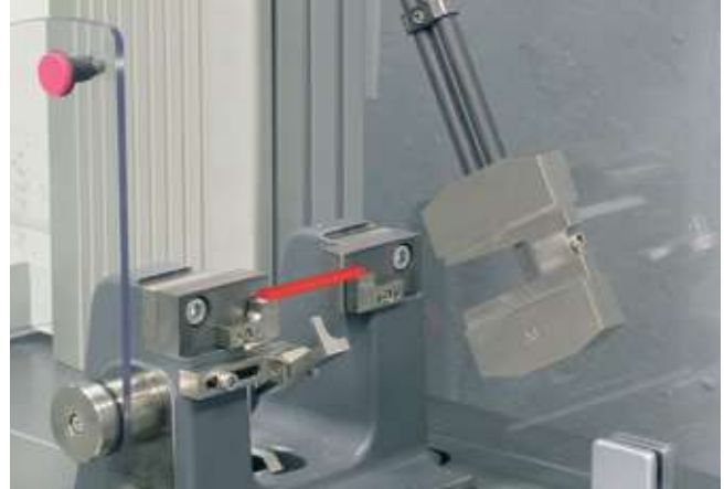
Fig. 1: Notch alignment unit on a Charpy fixture
