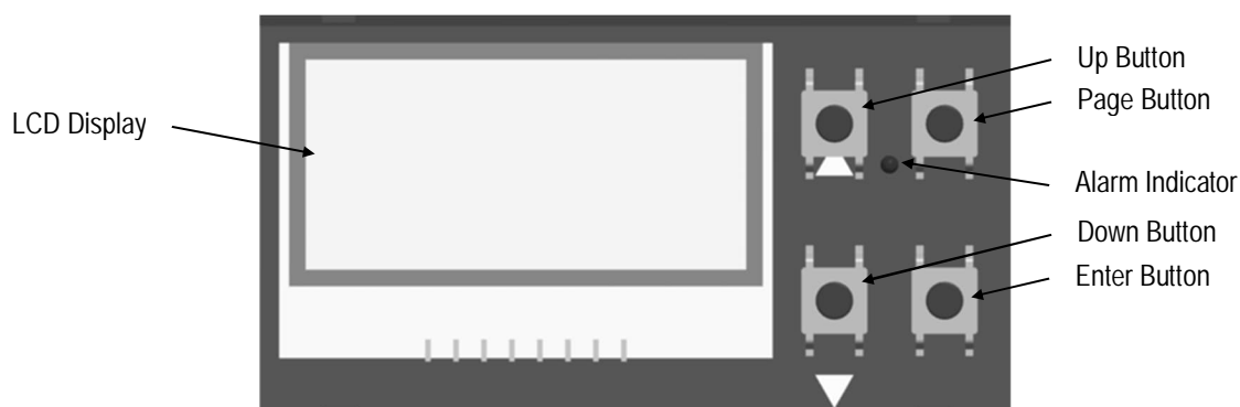
Figure 33: Control Panel for the Comm Box (DIN)
