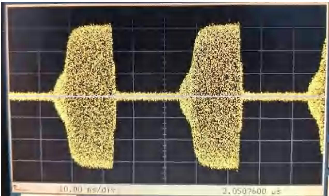
• Internal Pulse Modulation (38.8 GHz, 15ns period, 7 ns pulse width)
