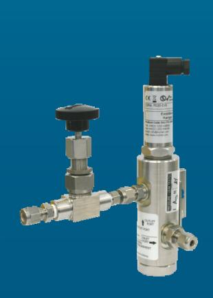
97109 Issue 3.1 October 2013 The Easidew Sampler is a modular low-cost, self-contained, filtration block and flow control arrangement which is suitable for any Michell impedance dew-point transmitter with 5/8" - 18 UNF process connection size, and is able to perform dew-point measurements at 200 barg (2900 psig).
