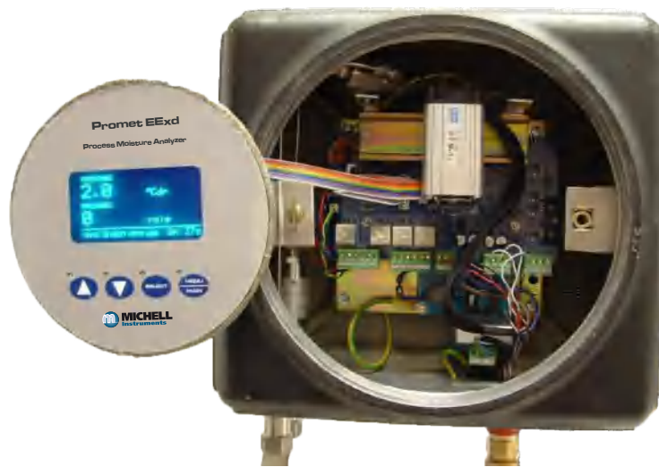
Figure 23 Ribbon Cable Connection
