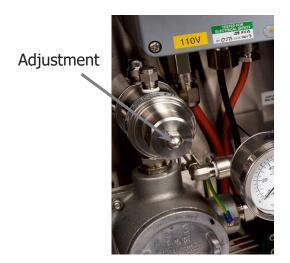
Figure 8 PR1 Adjustment Point
