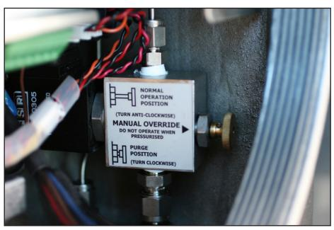
Figure 7 Solenoid Valve Location
