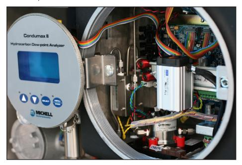
Figure 6 Removal of Interface/Display
