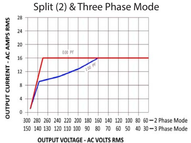
Short term overloads to 20A are permitted. Operating time before thermal shutdown or circuit breaker trip varies from seconds to several minutes depending upon line and temperature conditions.
