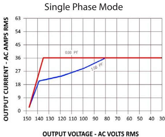
Short term overloads to 60A are permitted. Operating time before thermal shutdown or circuit breaker trip varies from seconds to several minutes depending upon line and temperature conditions.
