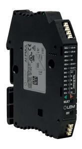
The universal Rogowski coil integrator Al-PMUL complements LEM's flexible clip-around coil ART and ARU range. The design is based on digital processing to give combined dynamic range, accuracy and versatility of use. It offers a wide range of output signals both RMS and instantaneous. Al-PMUL is DIN rail mounted and can be stacked for multiphase application without spacing thanks to its low power dissipation.
