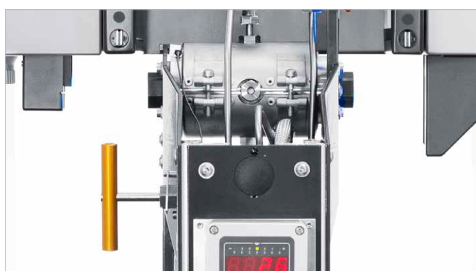
Sample positioning with closed pressure chamber.
