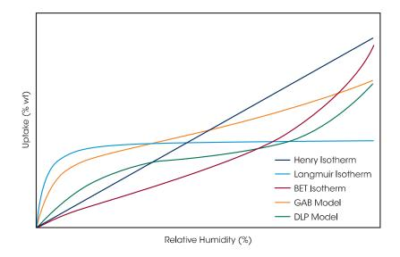
In a simple-to-apply procedure, TRIOS software determines the parameters of the models to obtain a best fit between the experimental sorption data and the physical or empirical model. The modeling allows users to interpolate between and extrapolate data points as well as to determine isosteric heats of adsorption. Parameters of the physical models provide insight about characteristic properties of the material, such as kinetics of adsorption and BET surface area.
