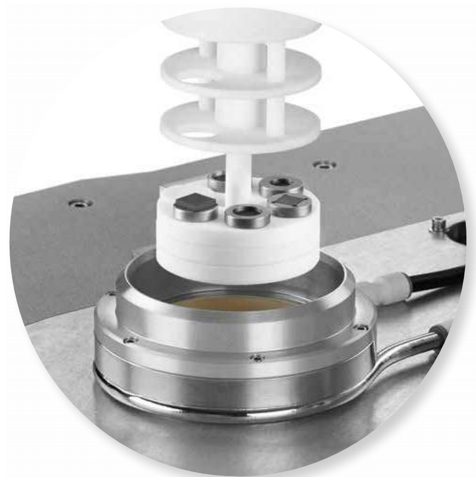
Patented Multi-sample Carousel with Flexible Tray and Adaptors
