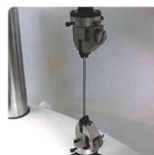
Testing of Tire Cord
