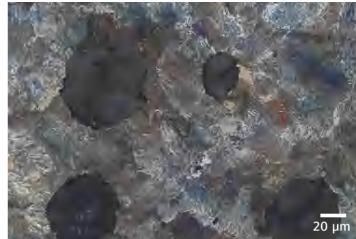
Cast iron, brightfield, objective: EC Epiplan-APOCHROMAT 50×/0.95
