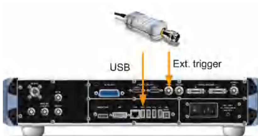
Figure 6-2: Connecting a power sensor for use as an external trigger
