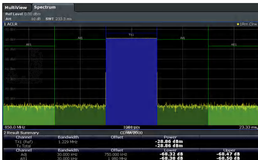
Figure 5-21: Measuring the channel power and adjacent channel power ratio for CDMA2000 signals with zero span (Fast ACLR)
