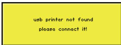
Connect the USB printer to the **connector for an external USB device** [17] and confirm the message by pressing the **ENTER key** [5].
