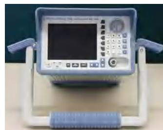
2. Slide the handle lengthwise while twisting it radially in steps of about 12°.
