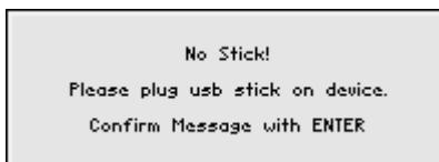
Connect the USB stick to the **connector for an external USB device** [17] and confirm the message by pressing the **ENTER key** [5].
