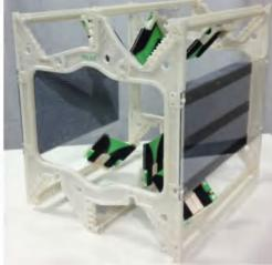
Figure 5-16: Antenna ring with six Vivaldi antennas, right: with two absorber brackets and absorbers
