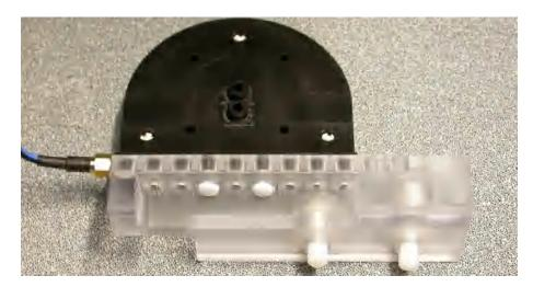
Figure 7-76: LF loop antenna fixed on the antenna holder
