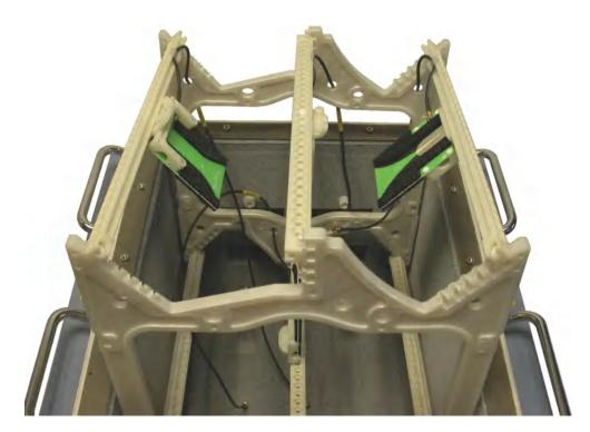
Figure 7-25: Take the full antenna ring out of the chamber
