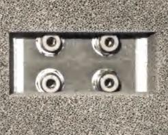
Figure 5-29: Pneumatic feedthrough with four push-pull valve connectors
