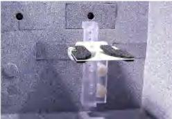
Figure 5-20: Antenna holder mounted inside the chamber at the rear wall with one Vivaldi antenna
