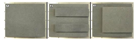
Figure 7-40: Different absorber material configurations on the inside of the top cover. In these pictures, the "FRONT" edge of the cover is on the right-hand side
