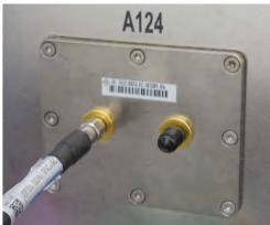
Figure 5-24: Twin RF feedthrough with two female PC 1.85 mm connectors
