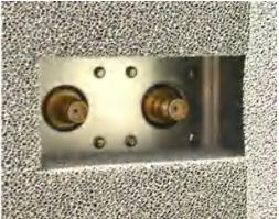
Figure 5-21: Two RF feedthroughs with N and SMA connectors
