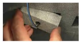
3. Use an SMA wrench to disconnect the antenna cables from the SMA connectors at the chamber's rear wall.
