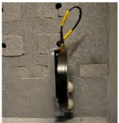
Figure 7-74: LF loop antenna mounted in RF Shielded Box (two of various possible positions)
