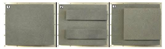
Figure 7-77: Different absorber material configurations on the inside of the top cover. In these pictures, the "FRONT" edge of the cover is on the right-hand side
