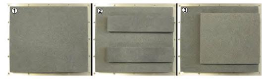
Figure 7-70: Different absorber material configurations on the inside of the top cover. In these pictures, the "FRONT" edge of the cover is on the right-hand side
