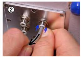
Figure 5-30: Handling pneumatic tubing with the push-pull connector
