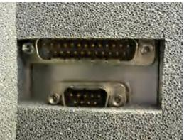
Figure 5-25: Feedthrough with 25-pin and 9-pin D-Sub connectors
