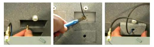
Make sure to make a note of the allocation of which SMA connector the antenna is connected to.
