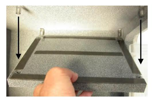
**Note**: It may be a bit difficult to detach the absorber sheet from the spacer in the lower corner, close to the door. In this case, try to squeeze your fingers between the absorber sheet and the absorber material on the chamber's ground, to be able to pull from underneath.
