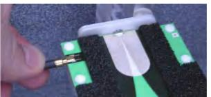
Figure 7-47: Connecting an antenna
