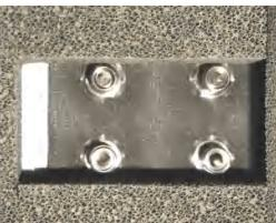
Figure 5-28: Fiber-optic feedthrough with four FSMA connectors
