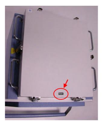
Figure 7-5: Top cover with sticker indicating the cover's front edge
