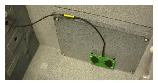
Figure 5-38: One narrowband antenna mounted in a low position on the right chamber wall
