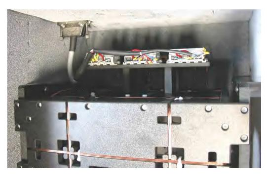
Figure 5-44: View from above (top cover opened): wiring board, cables and connector
