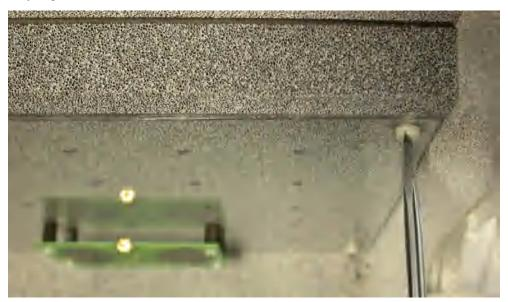
8. Remove the acrylic glass sheet and the absorber sheet from the chamber's wall.
