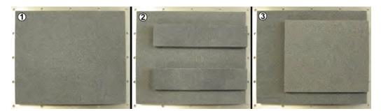
Figure 7-48: Different absorber material configurations on the inside of the top cover. In these pictures, the "FRONT" edge of the cover is on the right-hand side
