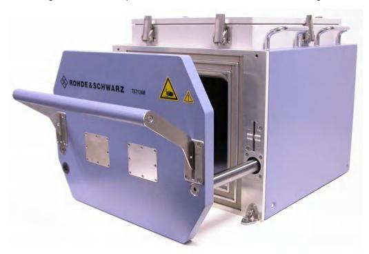
Figure 1-1: RF Shielded Box with front door / drawer opened
