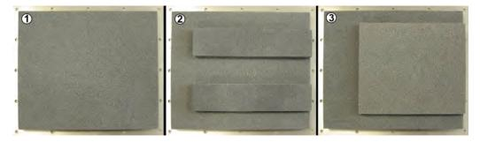
Figure 7-23: Different absorber material configurations on the inside of the top cover. In these pictures, the "FRONT" edge of the cover is on the right-hand side
