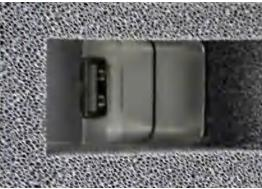
Figure 5-26: Filtered USB 2.0 feedthrough
