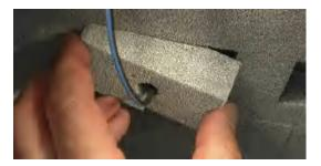
3. Use an SMA wrench to disconnect the antenna cable from the SMA connector at the chamber's rear wall.
