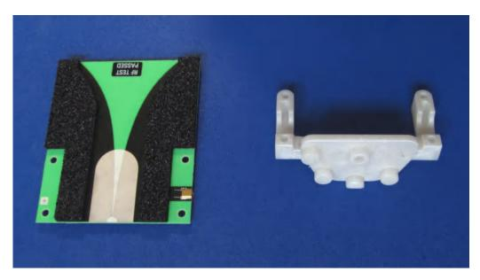
Figure 5-12: One of the Vivaldi antennas and its fixture
