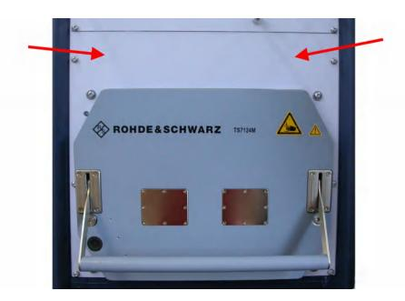
Figure 5-48: RF Shielded Box fixed in a 19" rack by the rack mounting kit
