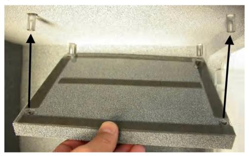
Installation of Narrowband Antennas
