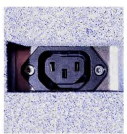
Figure 5-31: Electric power feedthrough
