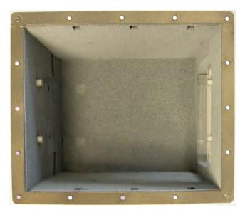
Figure 5-1: Empty chamber with basic absorber material (seen from top, cover removed)
