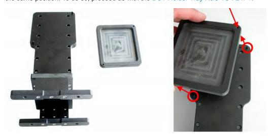
Figure 5-46: DUT holder with door mounting kit (left) and DUT tray (center), the assembly is shown on the right (two pins match two holes in the tray)
