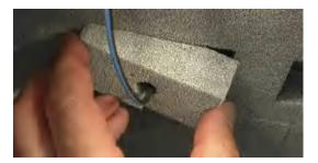
10. Connect the 20 cm SMA/SMP cable, delivered with the Antenna Holder R&S TS-F24-AH2, to the SMP connector at the antenna:
