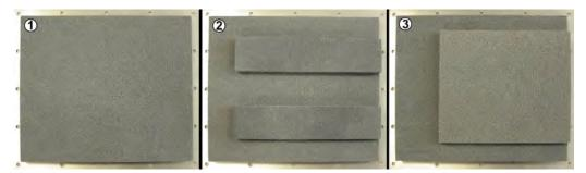
Figure 7-4: Different absorber material configurations on the inside of the top cover. In these pictures, the "FRONT" edge of the cover is on the right-hand side
