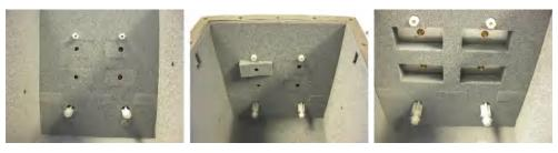
Figure 7-36: Remove detachable absorber pads from the rear wall, as required
