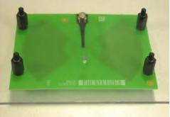
If you mount the antenna next to the lower edge of the acrylic glass sheet (close to the chamber's ground), orient this antenna's SMP connector pointing away from the edge. Hence, let the SMP connector point upwards, as the lower antenna in Figure 7-65 and Figure 7-63.
