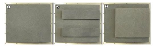
Figure 5-2: Different absorber material configurations on the inside of the top cover. In these pictures, the "FRONT" edge of the cover is on the right-hand side
