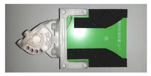
Figure 7-58: Antenna on fixture and 45° adapter, tilted at  $\gamma$  = +45°
