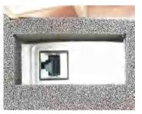
Figure 5-27: Gigabit Ethernet feedthrough for a LAN connection
