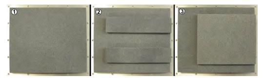
Figure 7-73: Different absorber material configurations on the inside of the top cover. In these pictures, the "FRONT" edge of the cover is on the right-hand side
