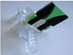
Figure 7-42: Two views of the antenna holder with one antenna mounted
