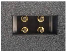
Figure 5-22: Four RF feedthroughs with SMA connectors
