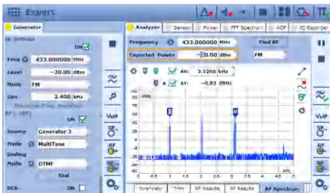
The multitone generator generates up to 20 tones.
