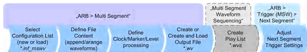
Figure 4-27: Basic workflow for generation of multi-segment waveforms
