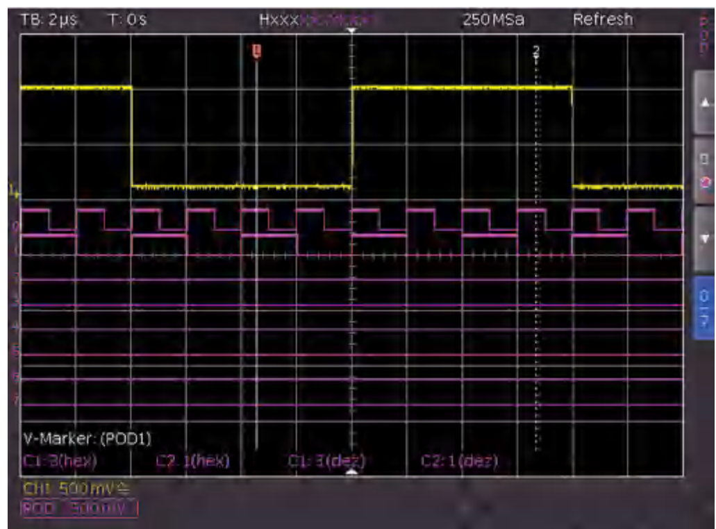
Figure 10-2: Logic channels: display settings
