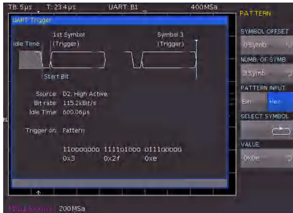
Figure 12-13: Trigger menu to trigger on a data pattern
