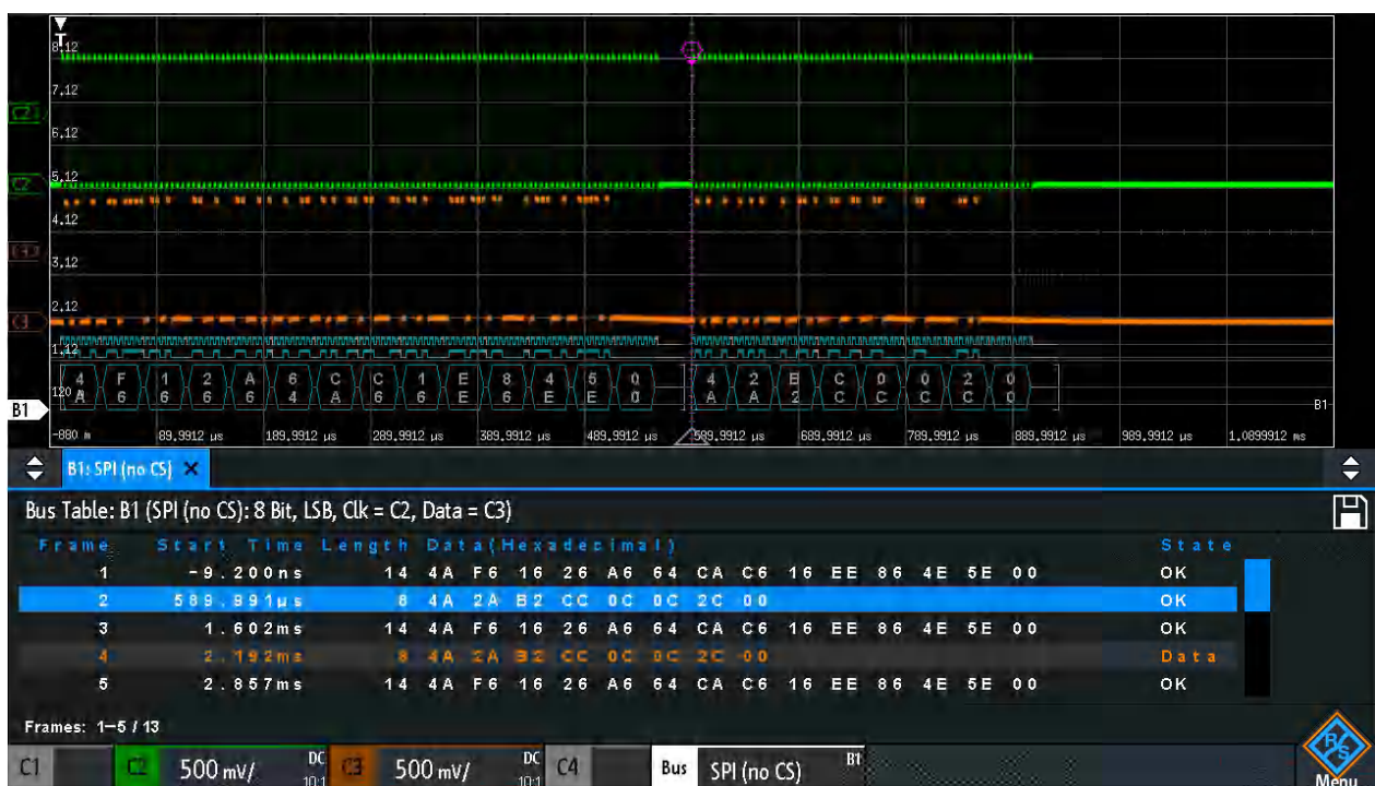
Figure 12-8: Decoded SPI (no CS) signal with Bus Table. The first frame has 14 words and the second has 8 words.
