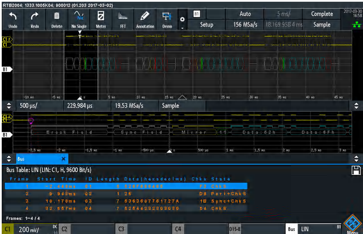
Figure 13-37: Decoded LIN signal with frame table and applied label list
