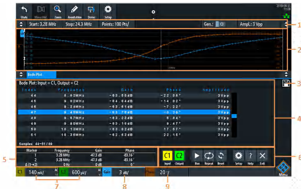
Figure 9-8: Bode plot display
