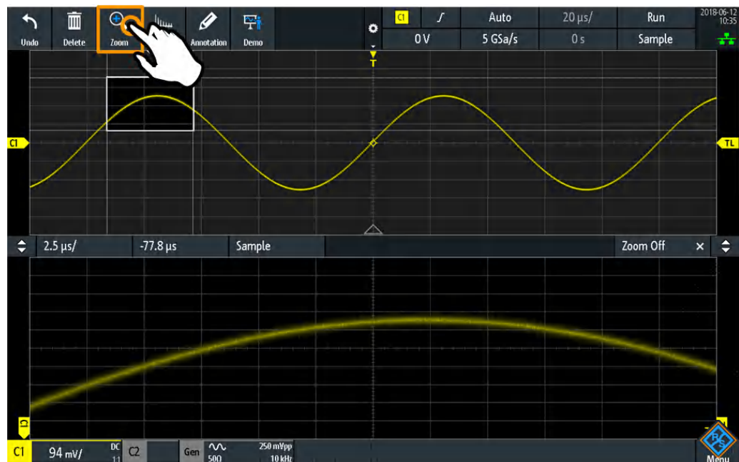
Figure 7-2: Display of vertical zoom
