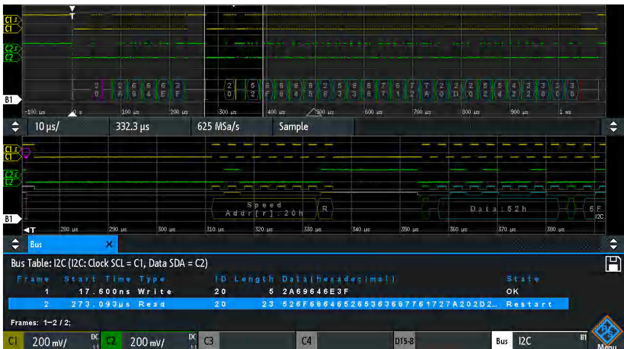
Figure 13-16: Decoded I2C signal with applied label list and zoom on second frame
