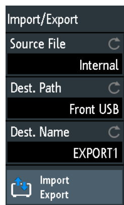
Import/export menu for instrument settings and equations
