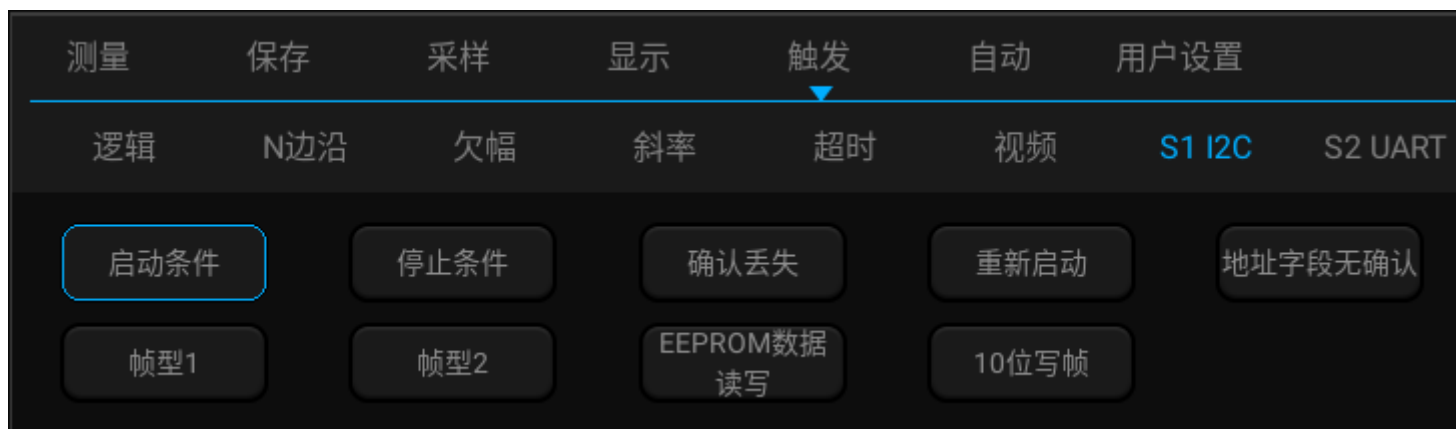
图13-23 I2C 触发方式配置菜单
