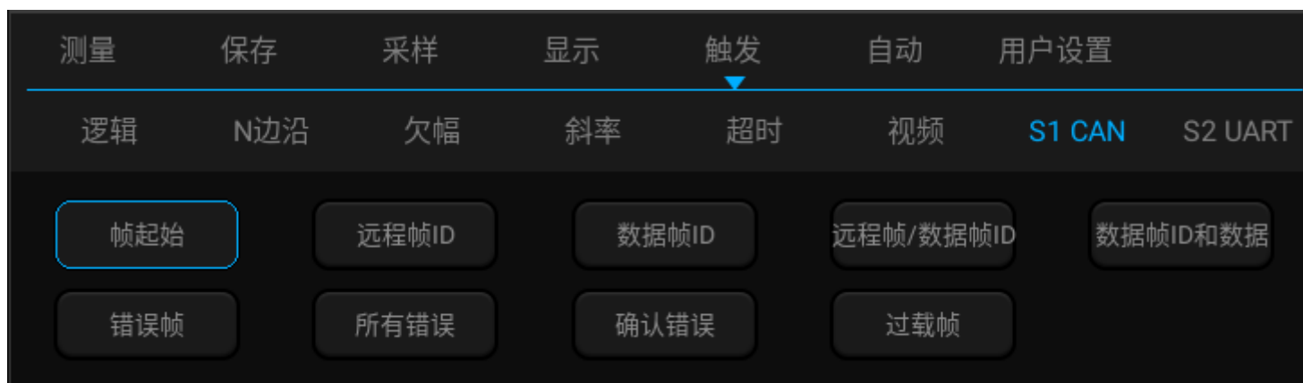
图13-15 CAN 触发方式配置菜单
