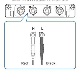
1 Connect the test leads to the banana jacks on the module.
