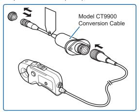
When Model CT9900 Conversion Cable is used, the instrument recognizes Model CT6846 or CT6865 (1000 A rating) as a 500-A AC/DC sensor. Set the conversion ratio to 2.00.
