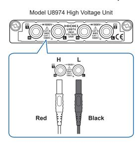
1 Connect the plugs of the connection cord to the banana jacks on the module.
