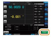
If measurement takes a long time, **[TRIG]** may be displayed as **[STOP]**. In this case, measurement can be suspended by pressing **[STOP]**.
