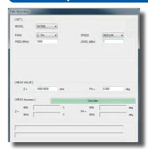
Basic accuracy can be calculated with the supplied application software.
