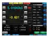
The LCR function allows you to measure the passive elements of capacitors and coils with a single measurement condition.
