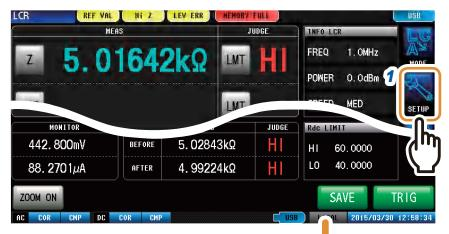
1 On LCR mode screen, press [SETUP] of the menu key.
