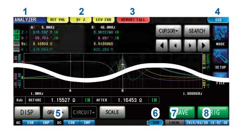
1 Displays the current measurement mode.
